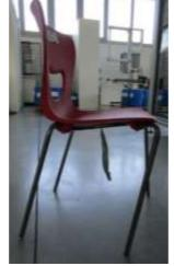
Detail of permanent deformation after test on one front leg
